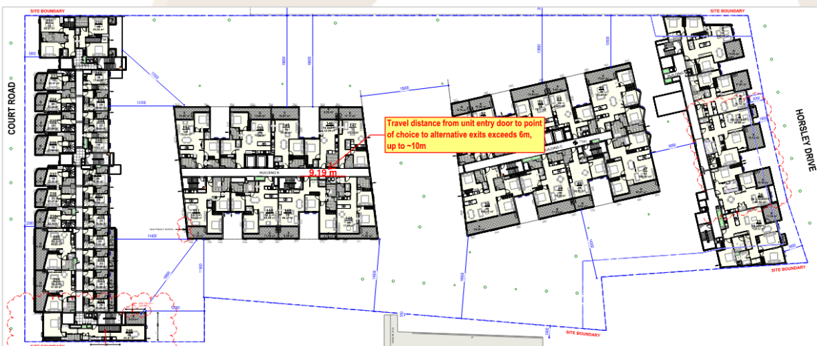
Figure 6.21 – Level 2 – 7 extended exit travel distances (typical)
